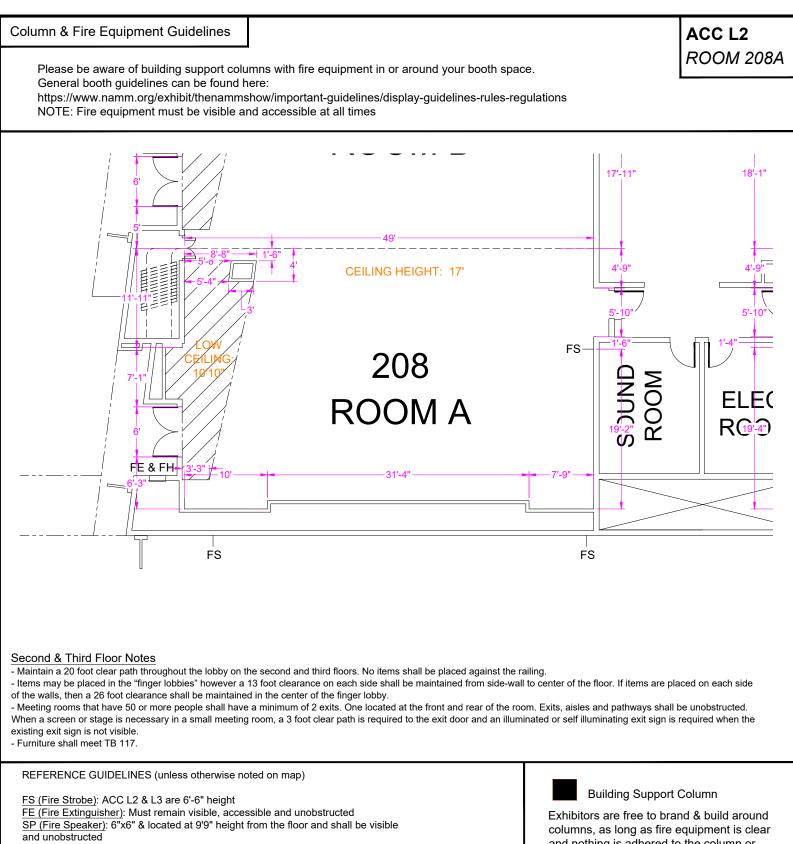
FH/FHC (Fire Hose Connection): Must remain visible, accessible and unobstructed FDR (Facility Door Release): Must not be blocked ES (Exit Sign): Located 9'-7" height unless noted otherwise. Must remain visible
